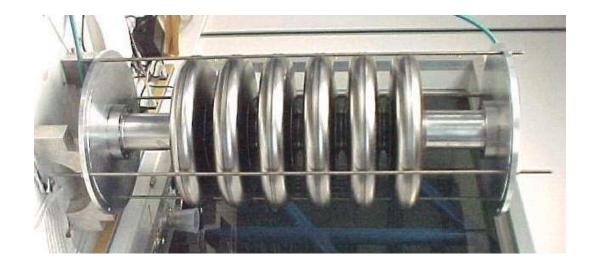
Figure 2.2. A 6-cell Niobium RF cavity.
