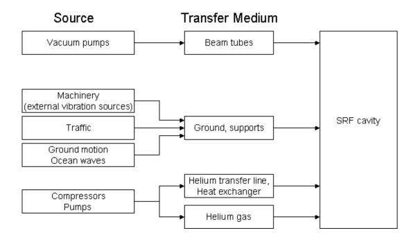
Figure 2.5. Possible sources and transfer mediums for microphonics [17].
